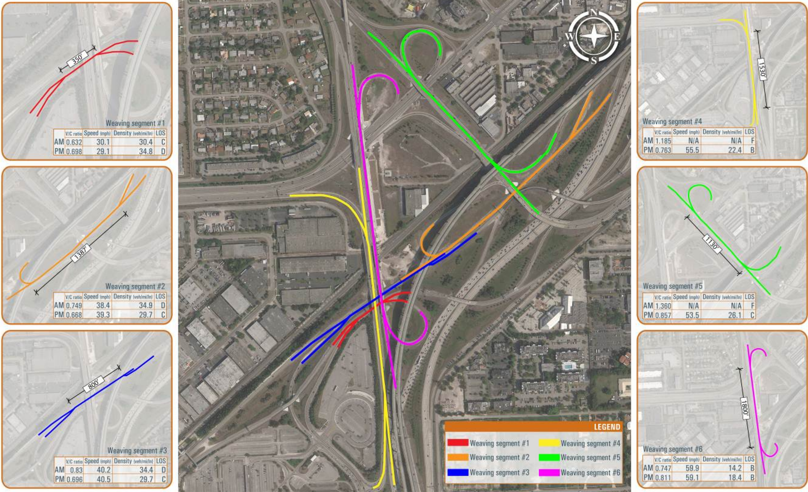
Figure 7-14 Weaving Analysis Results for Recommended-Build (2030)
