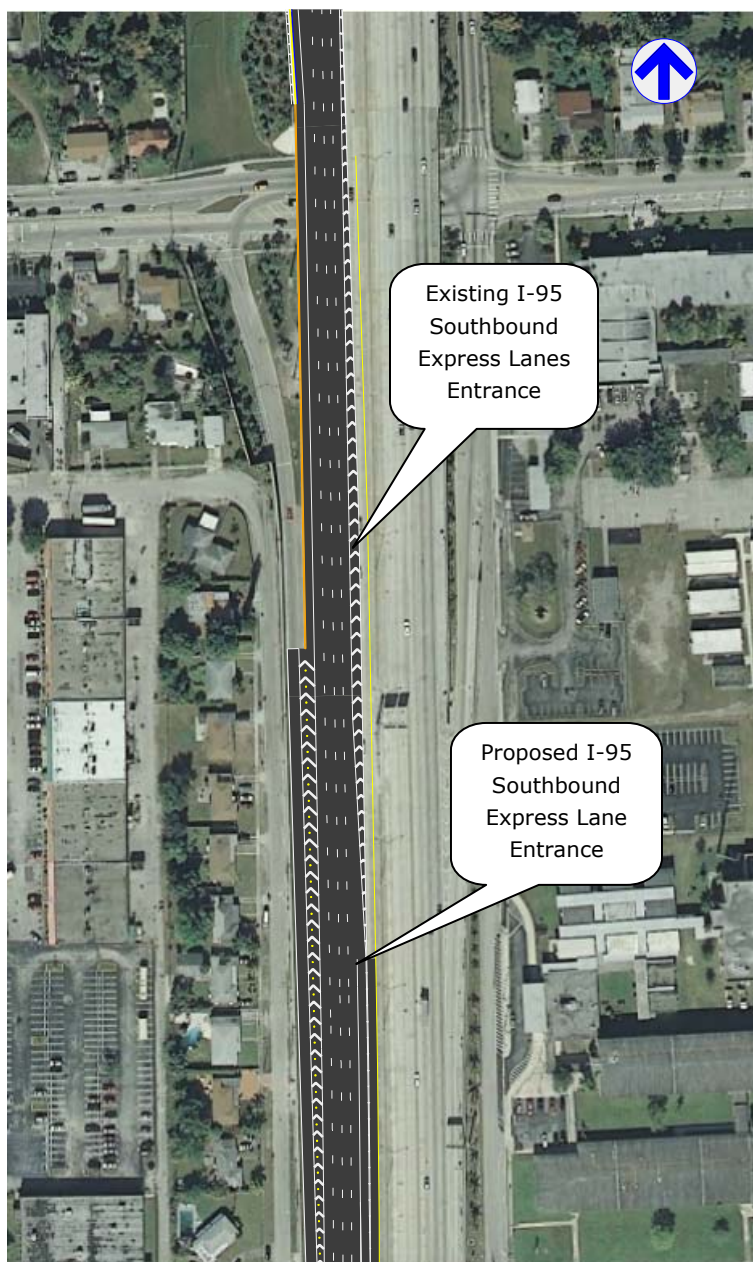
Figure 7-8 Relocation of I-95 Southbound Express Lane Entrance
