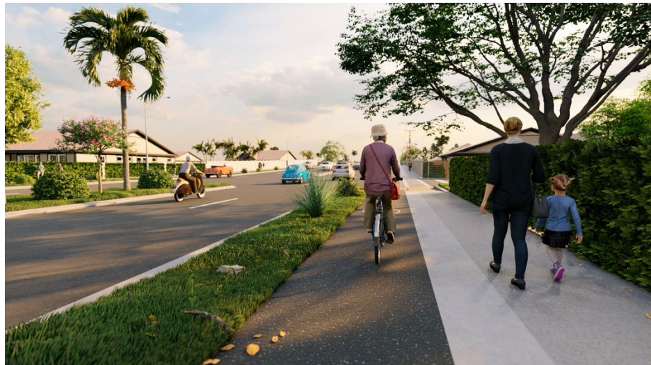
Figure 6-3 Sidewalk Level Separated Bicycle Lane
