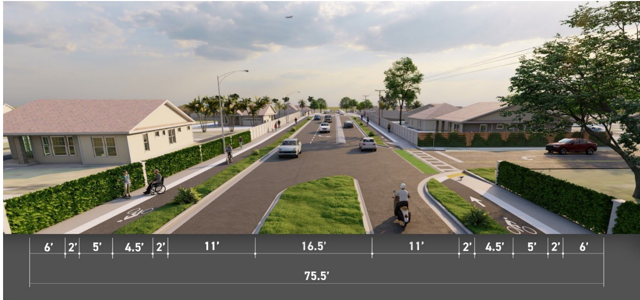
Figure 4-12 Build Alternative 1 Typical Section
