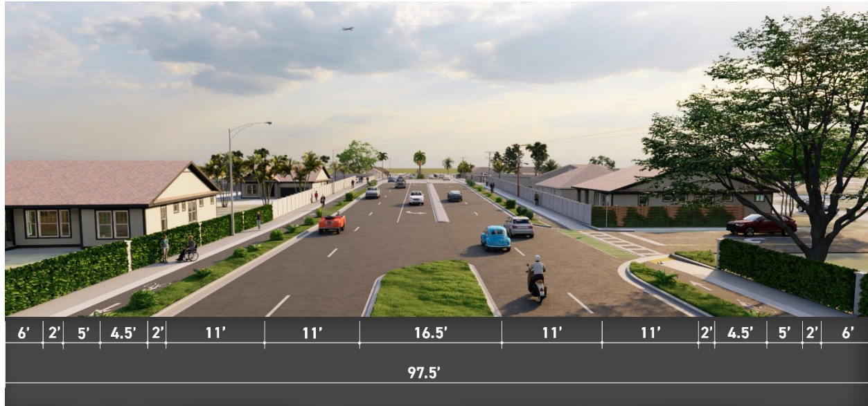
Figure 4-13 Build Alternative 2 Typical Section
