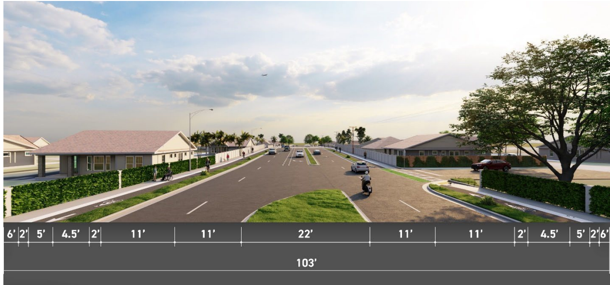
Figure 1-5 Build Alternative 3 Typical Section
