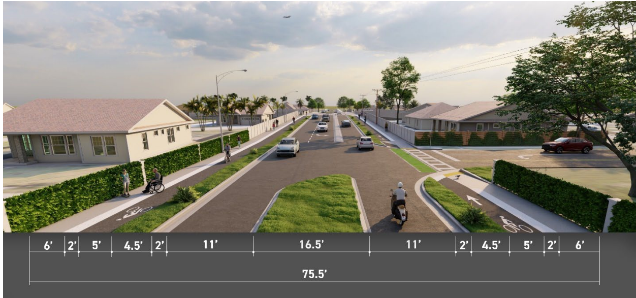
Figure 1-3 Build Alternative 1 Typical Section
