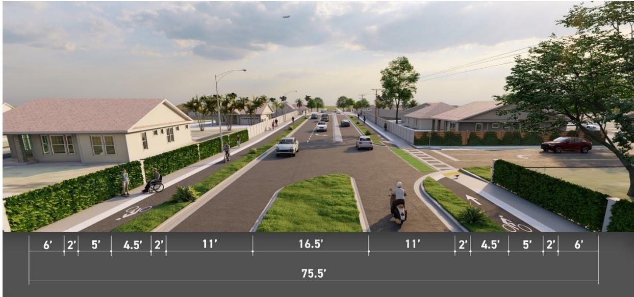
**Figure 4-12 Build Alternative 1 Typical Section**
