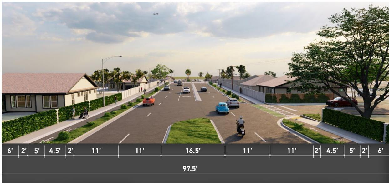
*Figure 6-1 Preferred Alternative Typical Section*
