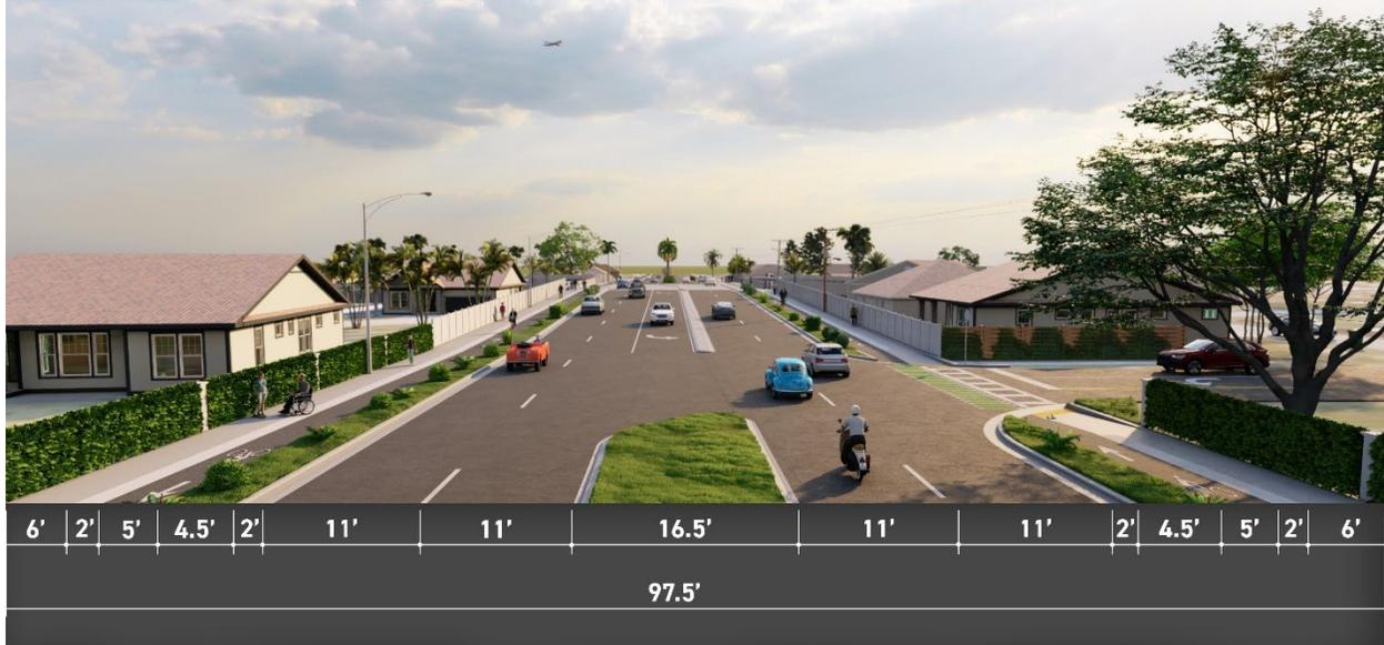
**Figure 4-13 Build Alternative 2 Typical Section**
