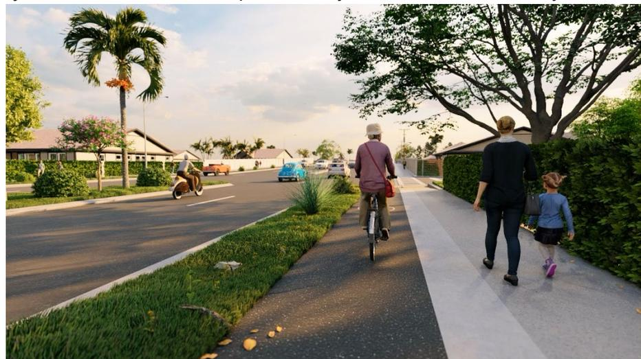
**Figure 6-3 Sidewalk Level Separated Bicycle Lane**
