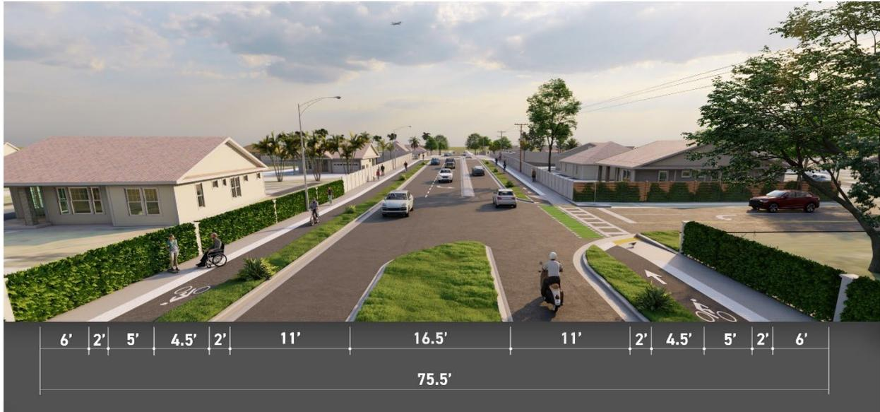
**Figure 1-3 Build Alternative 1 Typical Section**
