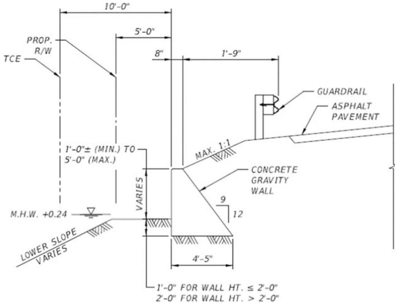
Attachment 2: Roadway Limits and Gravity Wall Excavation Depths from Conceptual Drainage Report
