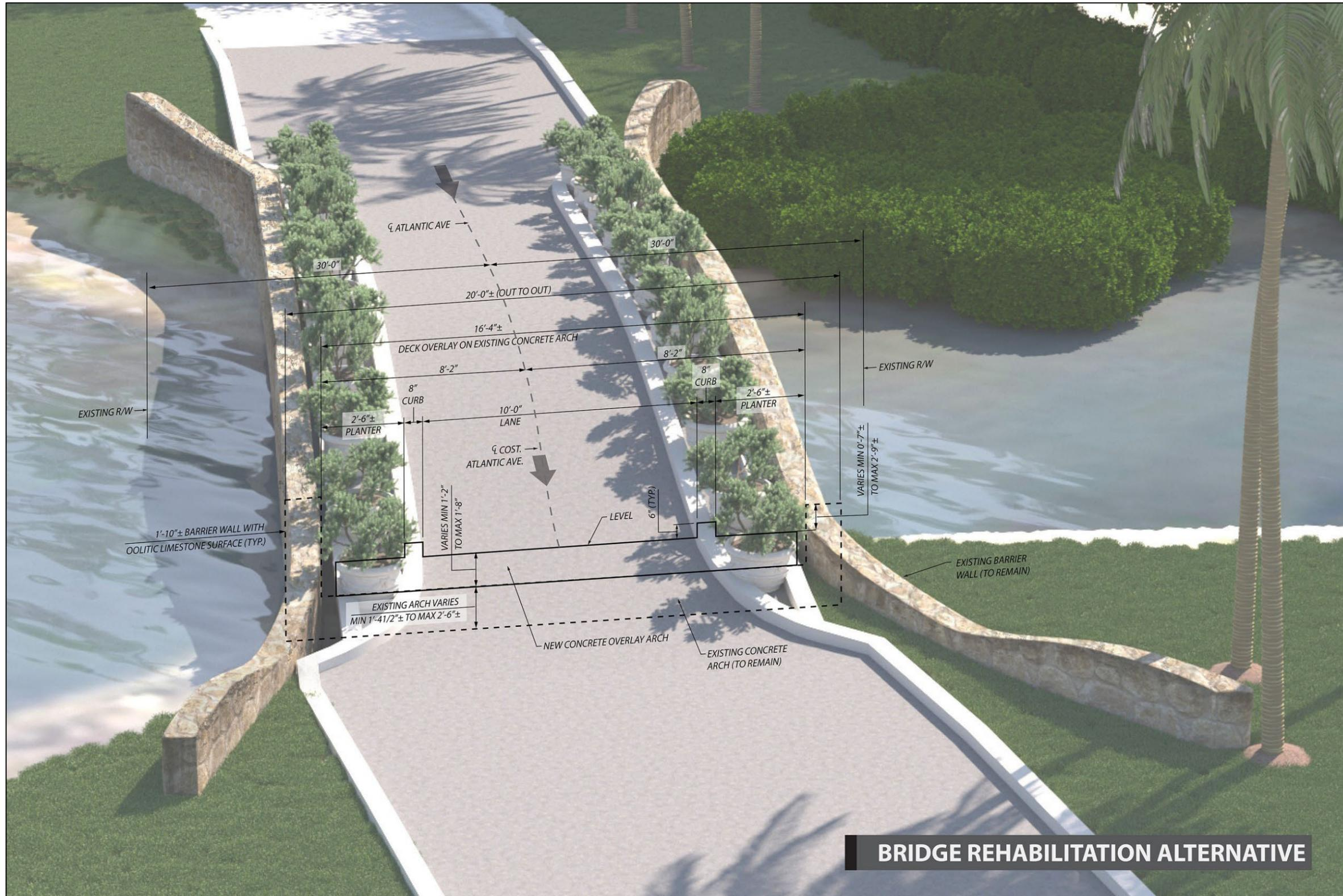
Figure 2-3: Rehabilitation Alternative (Build Alternative #1): Typical Section
