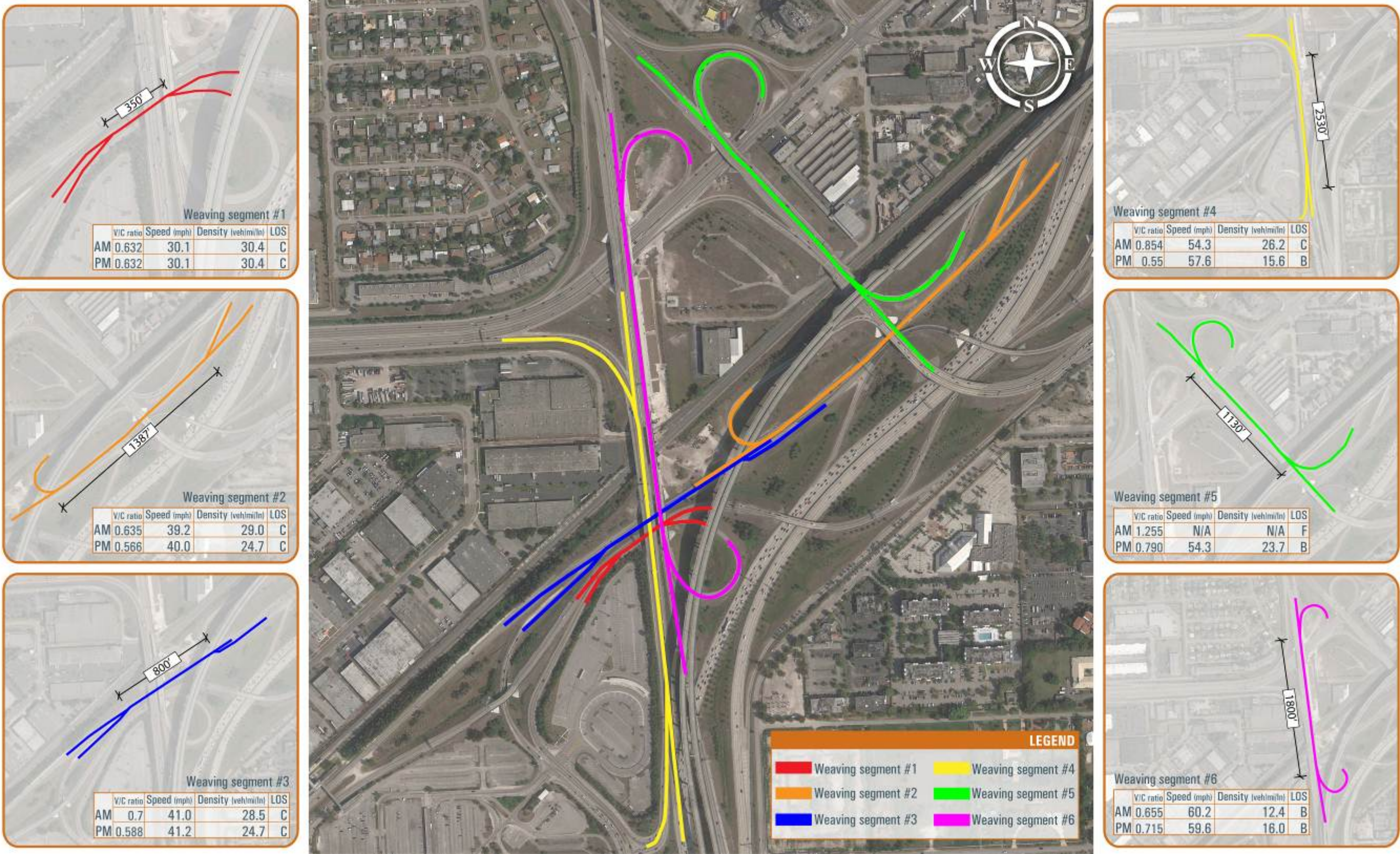
Figure 8-23 Weaving Segment Analysis –Build 3C 2018
