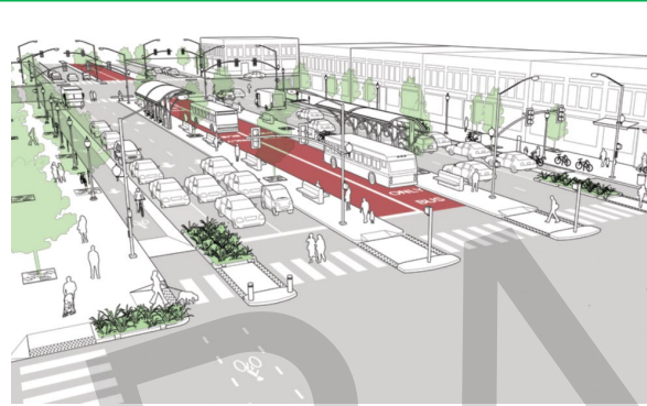
Source: NACTO guidance on median transitway (shown with one-direction separated bicycle lanes)
