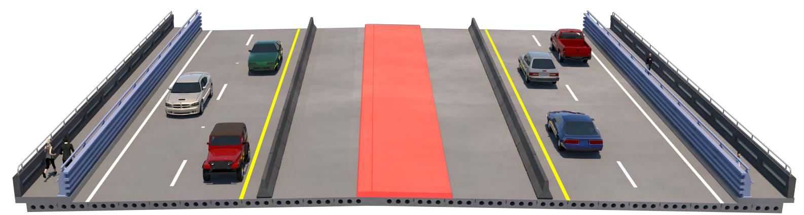
Remove the existing median and "close" the gap between bridges to allow a shift in traffic during future construction phases.
