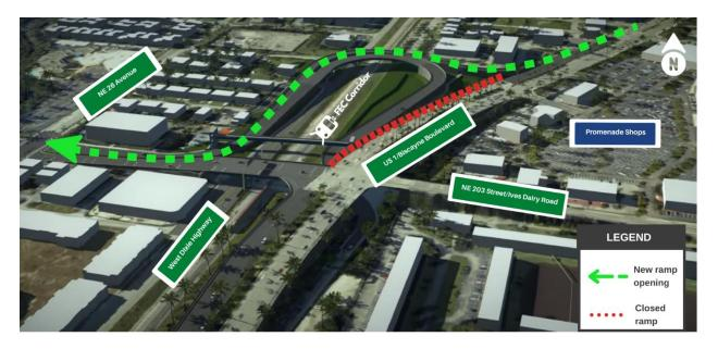
This new ramp marks a major milestone for the NE 203 Street Project. The ramp improves safety by removing vehicular traffic from crossing the FEC railroad tracks and onto the new flyover bridge ramp. It will also ease traffic flow for vehicles traveling through this critical intersection.
