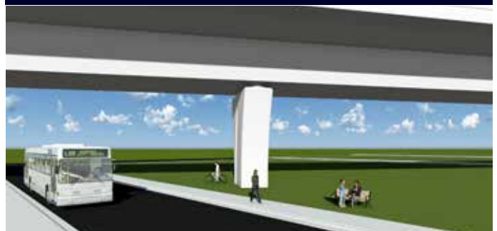
FIGURE 5: CONSTANT DEPTH BOX GIRDERS (AW-DMG)
