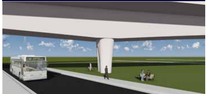
FIGURE 5: CONSTANT DEPTH BOX GIRDERS (AW-DMG)
